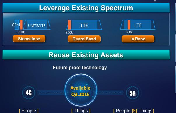
**More Connections** 1K -> 100K per cell **Deeper Coverage** 20+ dB gain over GSM **Low Power Consumption**
